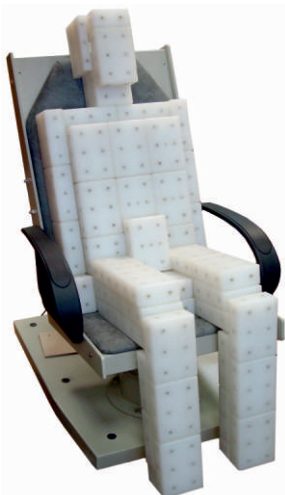
Whole body counter calibration using human body phantom
