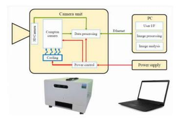
Its **exceptional sensitivity** (<1 nSv/h for an average level of natural radioactivity of ca. 300 nSv/h!) and **efficiency** allow the localization and the imaging of very low intensity radioactive sources with long exposures and those of intense sources very quickly.
