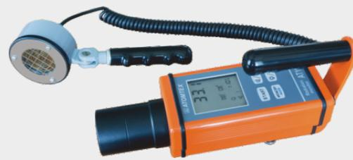
The Radiation Monitors can be delivered with an external BDPS-02 detection unit, designed for measuring alpha and beta particle flux density from flat contaminated surfaces, gamma and X-radiation ambient dose equivalent and ambient dose equivalent rate.
