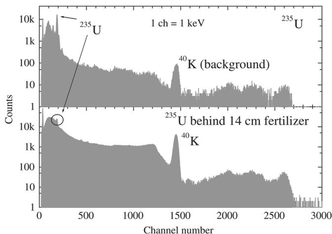
Fig. 8. The  $^{235}\text{U}$  spectra taken for the  $\text{LaBr}_3(\text{Ce})$  detector.
