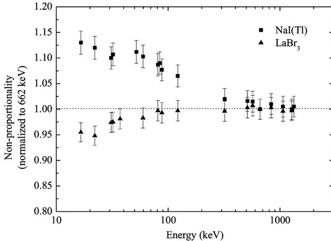
Fig. 1. A comparison of the nonproportionality curves measured for the  $\text{LaBr}_3(\text{Ce})$  and  $\text{NaI}(\text{Tl})$  ( $\varnothing 25 \times 31$  mm) crystals, respectively.
