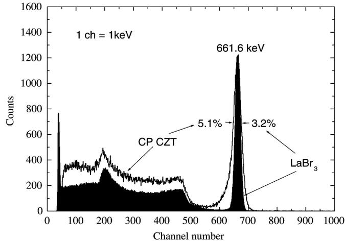
Fig. 3. The  $\gamma$ -ray spectra from a  $^{137}\text{Cs}$  source measured with  $\text{LaBr}_3(\text{Ce})$  and CP CZT.
