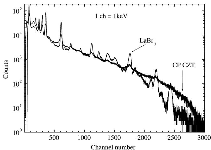
Fig. 7. The  $^{226}\text{Ra}$  spectra taken for the  $\text{LaBr}_3(\text{Ce})$  and CP CZT detectors.
