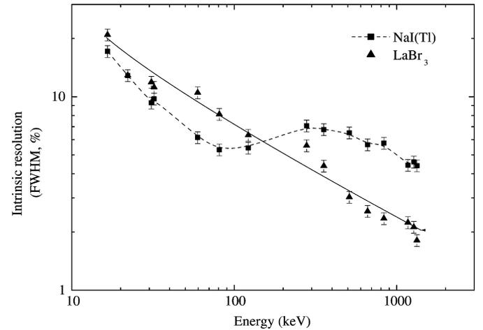
Fig. 5. The intrinsic resolution measured for  $\text{LaBr}_3(\text{Ce})$  and compared to  $\text{NaI}(\text{Tl})$  ( $\varnothing 25 \times 31$  mm).
