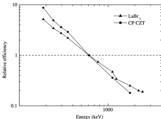
Fig. 6. Relative (to 609 keV) efficiency versus  $\gamma$ -ray energy determined for the  $\text{LaBr}_3(\text{Ce})$  and compared to  $\text{NaI}(\text{Tl})$  ( $\varnothing 25 \times 31$  mm).
