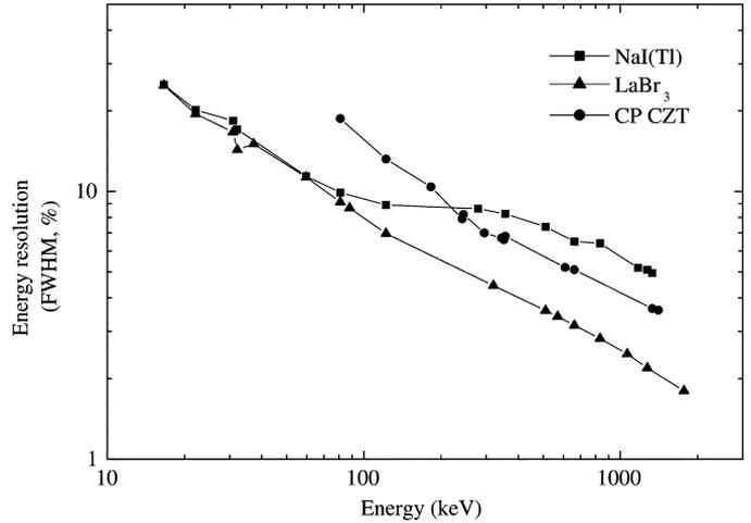
Fig. 4. The overall energy resolution measured for  $\text{LaBr}_3(\text{Ce})$  and CP CZT (compared to  $\varnothing 25 \times 31$  mm  $\text{NaI}(\text{Tl})$ ).
