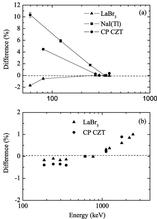
Fig. 2. Deviations from linearity measured with  $^{241}\text{Am}$  and  $^{133}\text{Ba}$  for the  $\text{LaBr}_3(\text{Ce})$ , CP CZT and  $\varnothing 1'' \times 1''$   $\text{NaI}(\text{Tl})$  detectors (a) and with  $^{226}\text{Ra}$  source for  $\text{LaBr}_3(\text{Ce})$  and CP CZT detectors (b). The error bars are of the data points size.
